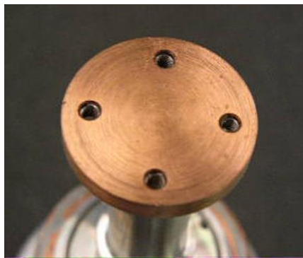
Figure 3-7. Four M4 Threaded Holes in the Cold Tip
