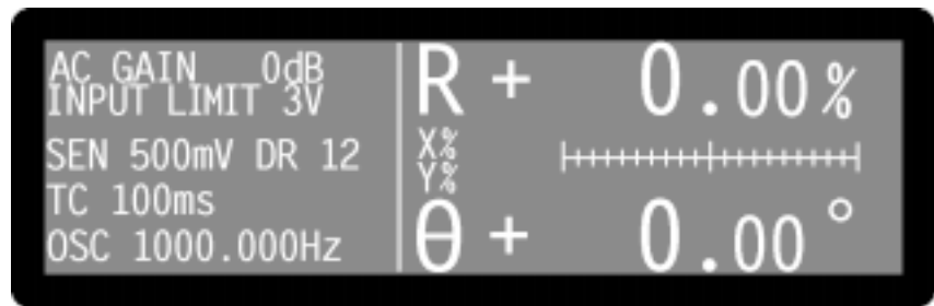
Figure 5-2, Main Display - Single Reference Mode
