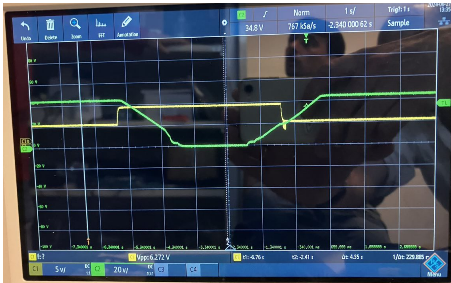
Figure 7: VSUB and one vertical clock as the erase procedure is performed
